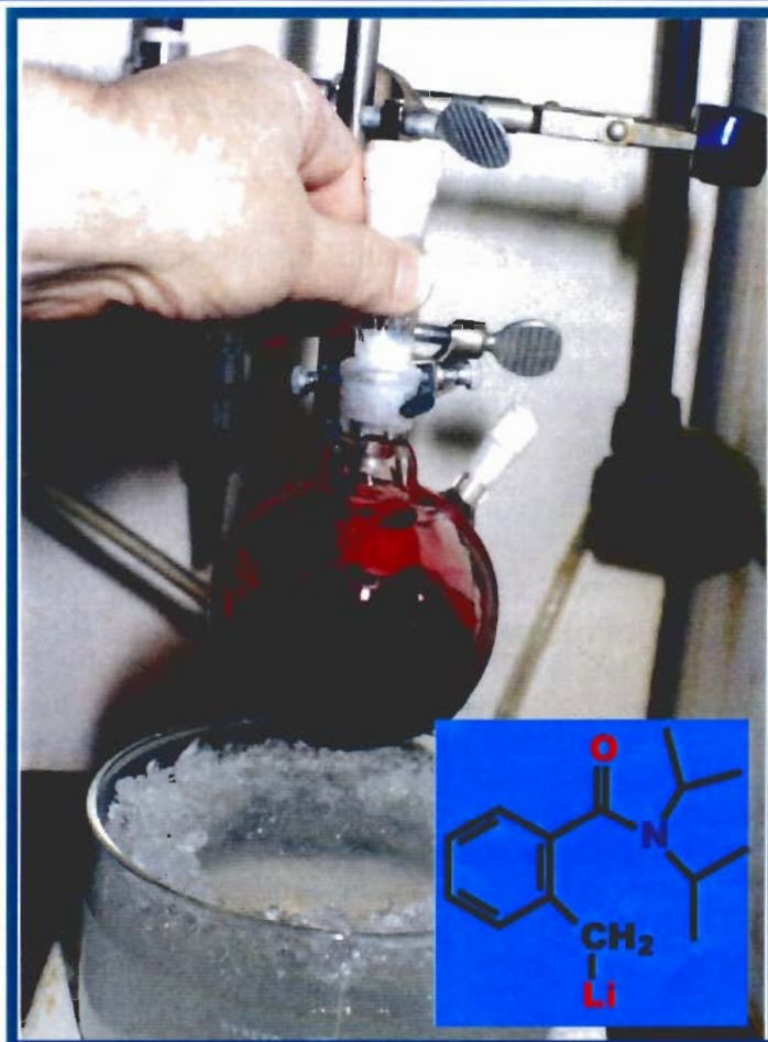
PHOTO 1: The amazingly intense and beautiful red-violet colour that is typical of an ortho-benzylic lithiated tertiarybenzamide. This solution is approximately 6 mmol of anion in 60 mL of THF. (Photo by Dr. Norman Reed, University College of the Cariboo)
